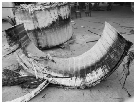
图3 C相电抗器第3包封 Fig. 3 The 3rd envelope of reactor of phase C
